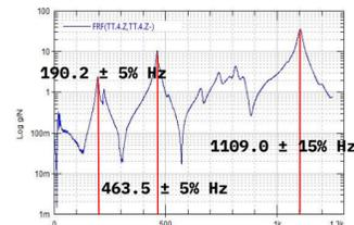
Fig. 5 Hammer Impact Test Results
