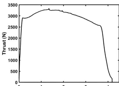
Fig. 2 Thrust (N) vs Time (sec) for static hot fire
