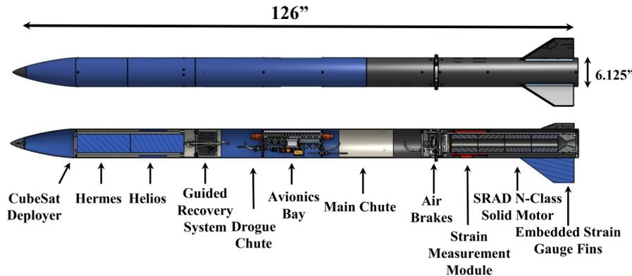
Fig. 4 External and internal view of Pitchfork with labels and principle dimensions
