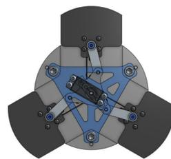
Fig. 8 Air Brake Top View
