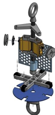
Fig. 3 GRAN exploded view housing not pictured
